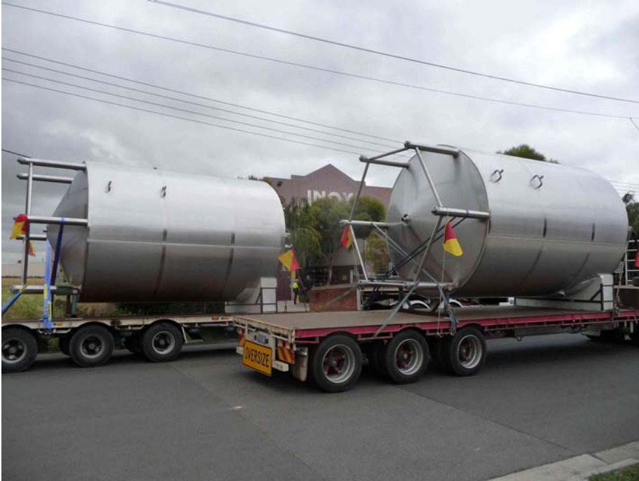
Bickfords 2 x 30,000L Alcohol Storage Tanks
