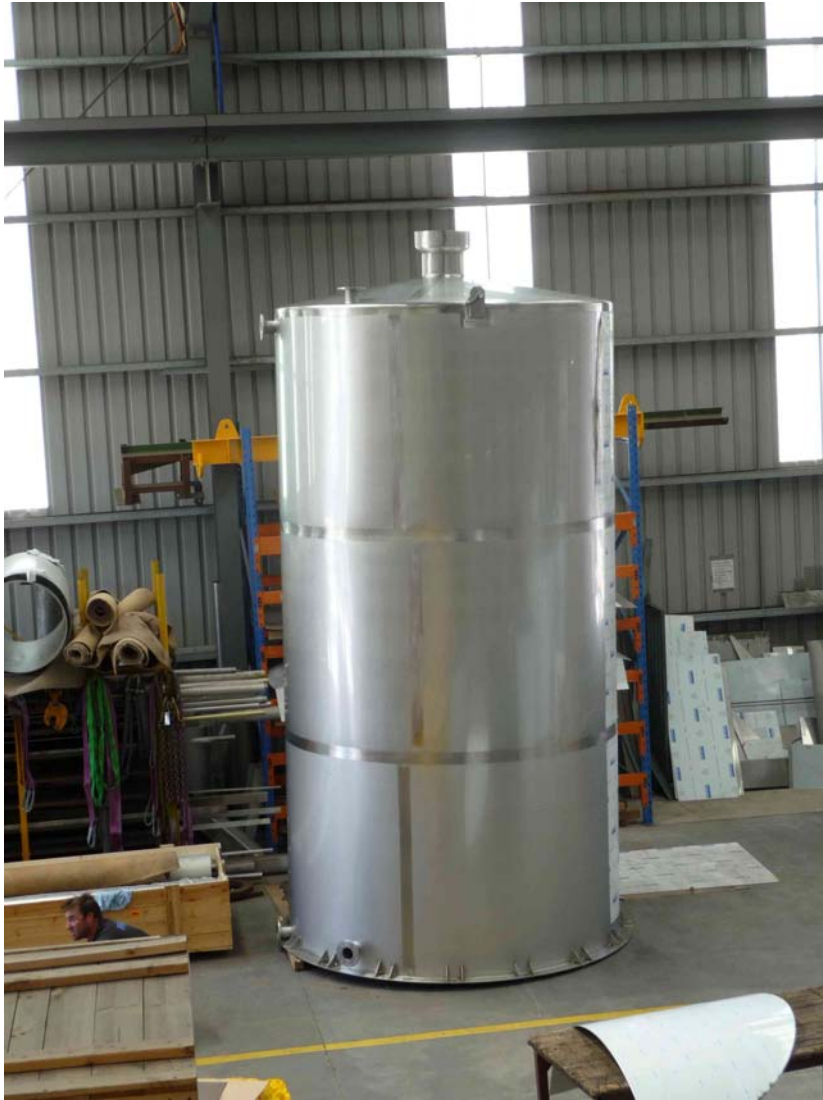
Murray Goulburn Cobram 25,000L Nitric Phosphate Tank
