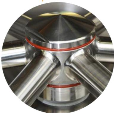
The hygienic design of the Kelstream ensures validated CIP cycles are successfully achieved between product batching.
